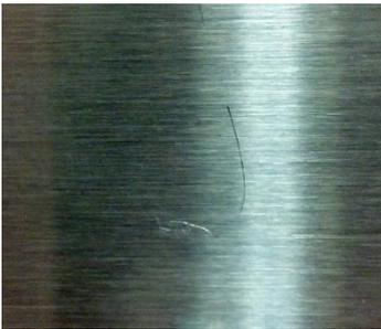
Before beginning work on the scratch, clean the surface of the stainless steel thoroughly to remove any dirt or oily film.
